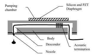
Figure 2. Schematic for new MEMs piezo ink jet.
